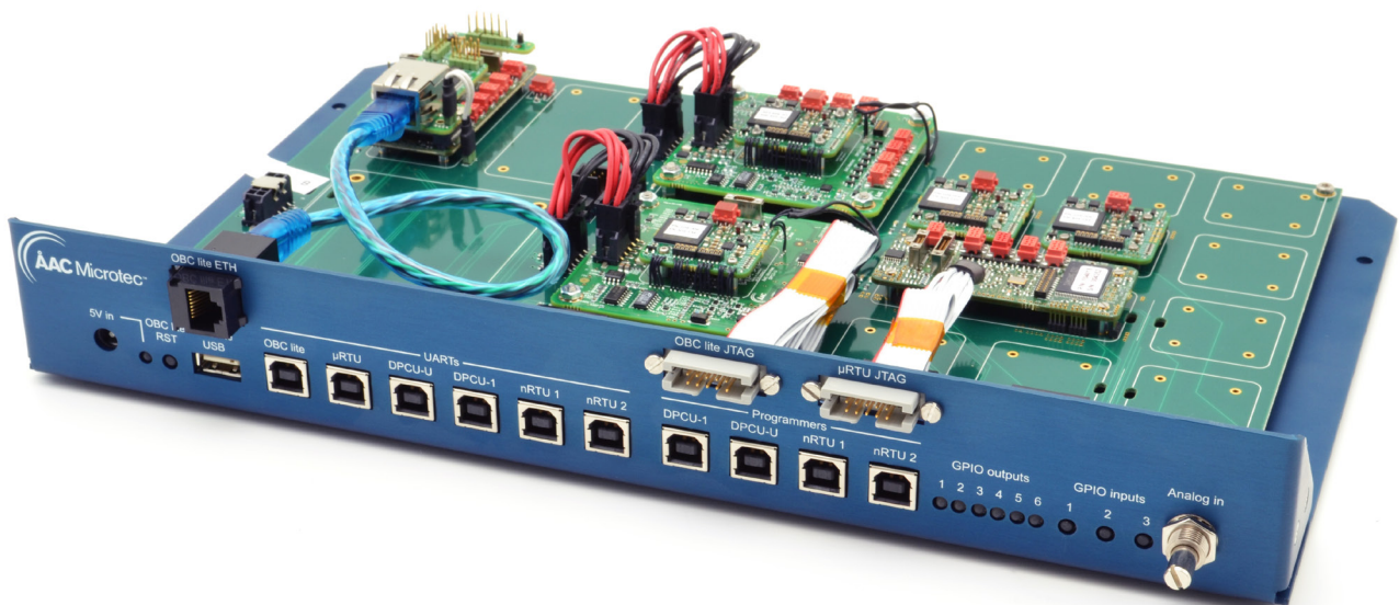
FIG. 1. Flat Satellite Development Kit products are assembled on top of the carrier board and connected to front panel interfaces for easy user access and operation.
